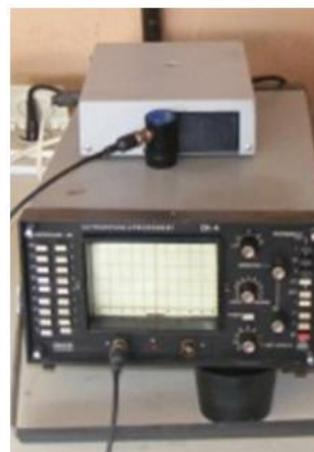
Type: **Electromagnetic generator / portable magnetostrictive Guided Wave** (Portable control, acquisition, processing, analysis and archiving data, including software acquisition, processing, analysis, evaluation and archiving data license).
