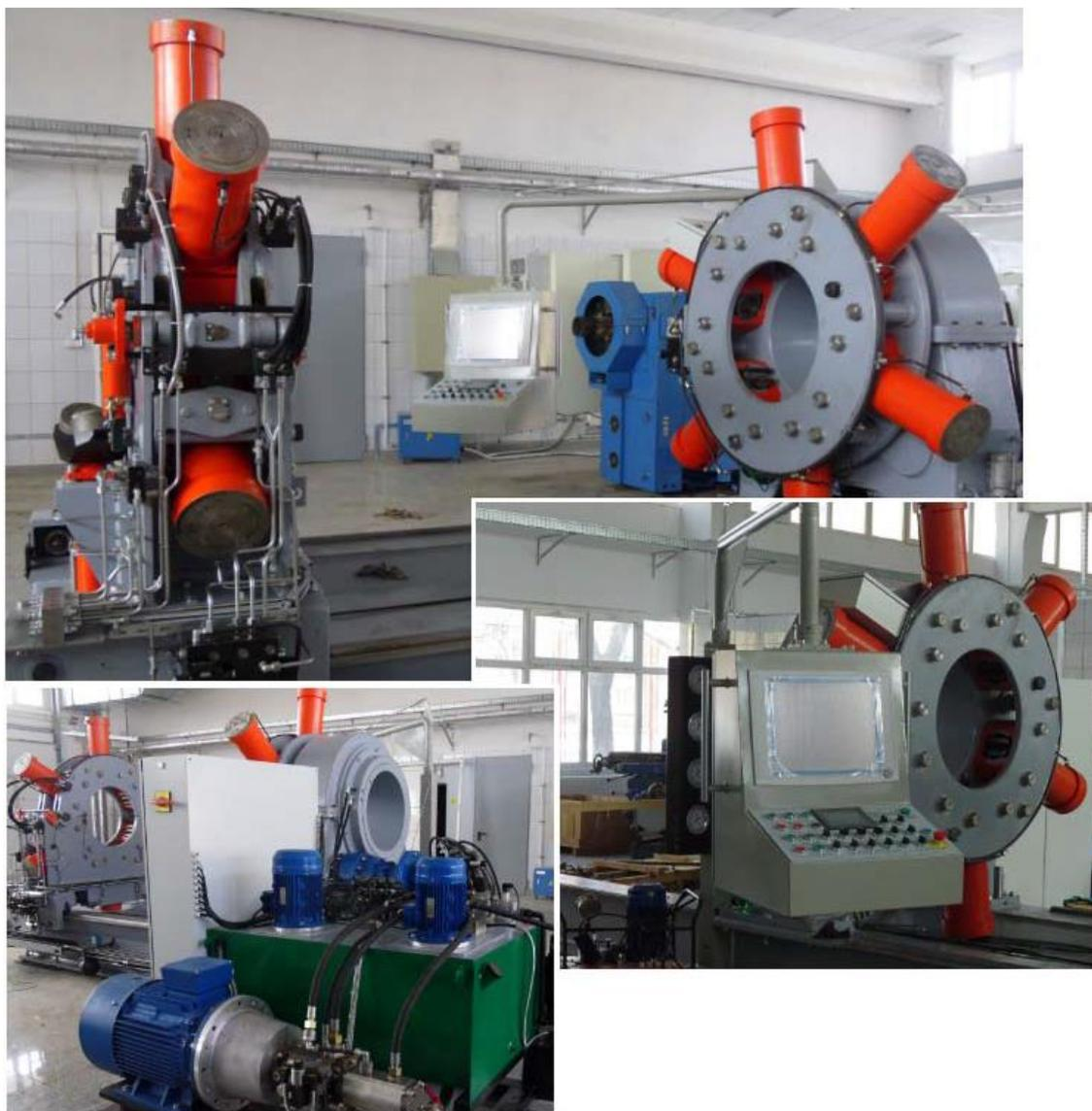
***2. Installation for traction testing 400 tf***
