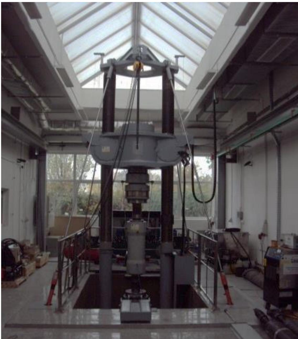
*3. Installation for external pressure (collapse) testing*
