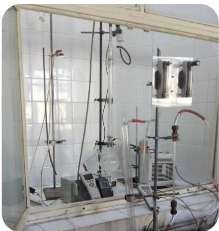
**Laboratory plant for carbon dioxide absorption**
