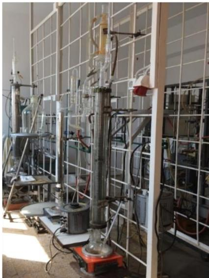
This distillation column is used to separate the various mixtures and advanced purification of some components.
