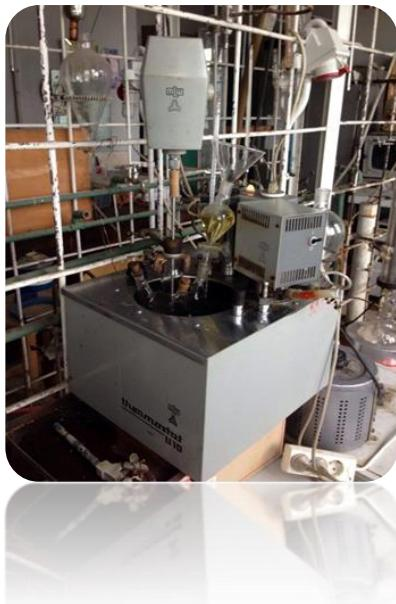
The installation is provided with a glass reactor placed in a thermostatic bath, with temperature and agitation rate control.
