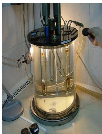
The plant includes a glass distillation column with bell-trays, allowing visualization of the distillation process, with reflux ratio and temperature control system, depending on the desired qualities for distilled products.
